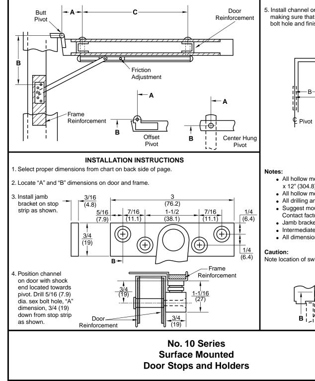
5. Install channel on door with "A" dimension sex bolt. Locate "C" dimension sex bolt hole making sure that channel is horizontal and parallel with stop strip. Drill 5/16 (7.9) dia. sex bolt hole and finish installing holder.
